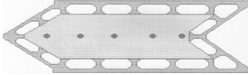
Fig. 3.4.1. Shiplike shape of pneumatic-type floating caisson
