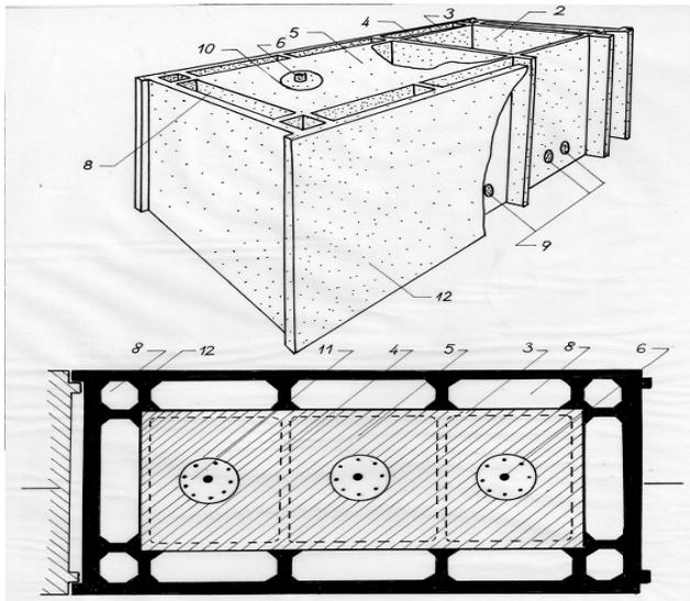
Fig.1.3. Prismatic pneumatic-type caisson
