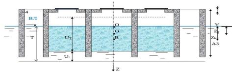
Fig. 4.1.1.1. Basic values of the equilibrium navigation of the caisson and coordinate system, determining its position relative to the water surface.
