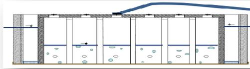
Fig. 3.4.4. Use of the caisson for capture of natural gas sources.
