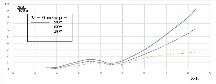
Fig. 4.3.4.6. The change in the frequency response of the keel oscillation by changing the angle of strike with the wave.
