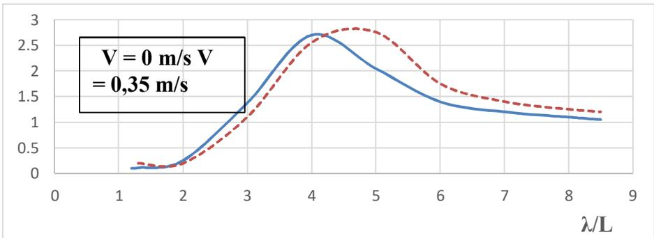
Fig. 4.3.4.2 presents the amplitude-frequency characteristics (frequency response) of vertical oscillation with and without
