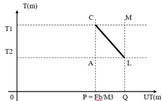
Fig. 4.1.2.2. Change of the draft of the caisson  $T$  depending on the size of the air column in the work chambers
