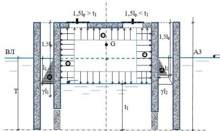
Fig. 3.5.1. Loads on the outer walls of the inner work chambers of the caisson.
