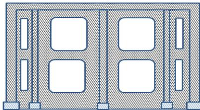
Fig. 3.4.3. Intermediate walls with large openings and thickening of the knives of the structure.
