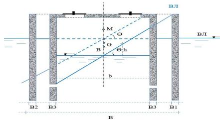
Fig. 4.2.4.1. Caisson resistances at large roll angles.
