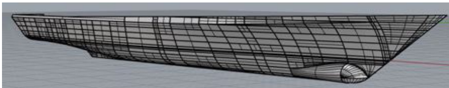
Figure 5. “Geometry with Big Parabolic Bulb”, bow profile
