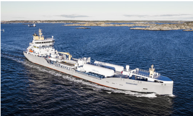
Figure 13. Forward location of the fuel tanks ( http://en.gh-lgm.com )
