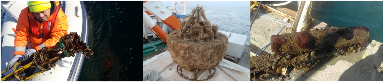
Figure 6. Bio-fouling of in situ sensors after three months
