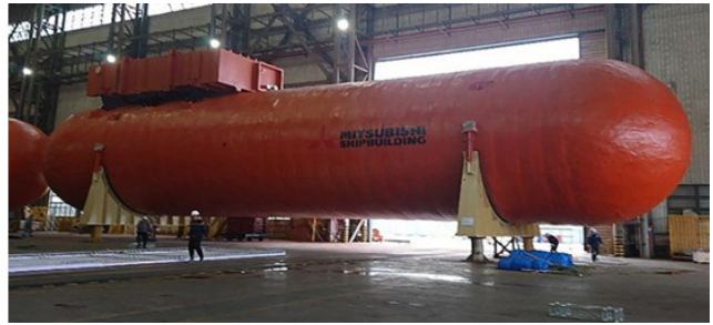
Figure 12. LNG fuel tank and the foundation ( https://www.jcnnewswire.co )
