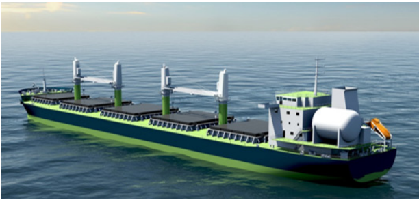
Figure 11. Aft ward location of the fuel tanks ( http://en.gh-lgm.com )
