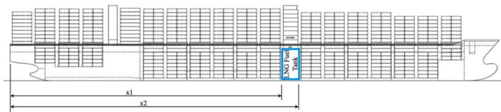
Figure 15. LNG fuelled containership and tank location [21]
