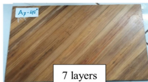
Figure 6. 7 layers laminated bamboo - fibreglass boards [8]
