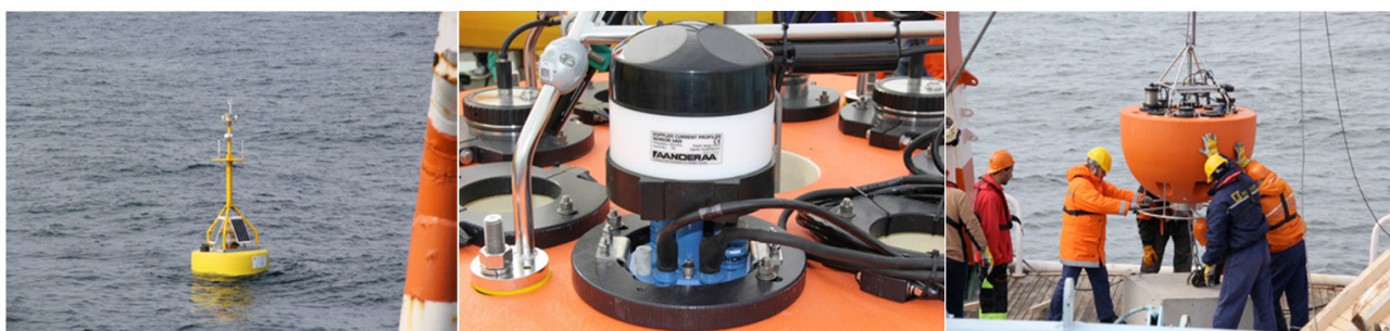
Figure 5. Deployment of moored buoy and bottom station in Varna bay
