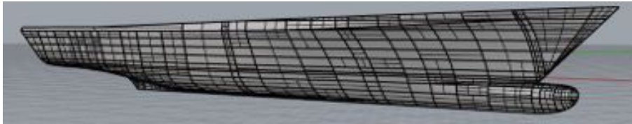
Figure 3. “Original hull”, bow profile
