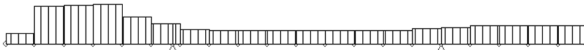
Figure 8. Ship lifting points at frames 73 and 25. Reaction at frame 73 - 431 t, at frame 25 - 213 t.
